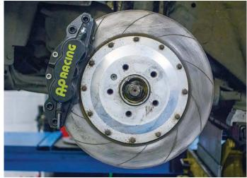
with Irmscher eighteens means that there's less than a Rizla paper's width of clearance between caliper and rim! 'Night and day' is a term of
