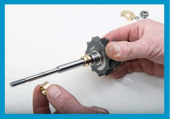
the cutout of the 270° thrust bearing, a special two-piece thrust collar is required (one piece fitting either side of the 360° bearing). This adds cost and complexity to production, but will offer increased potential for extra boost. As an example, the forced induction specialists at Turbo Performance say that a Garrett T3 will safely produce around 10psi of boost with a standard 270° thrust bearing in place, yet the same turbo will kick out as much as 30psi with a 360° bearing fitted. Crikey!
