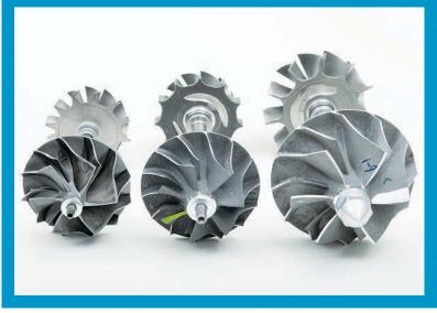
Now we're at the business end of your turbocharger! As we just mentioned, inside the unit's compressor housing is its compressor wheel. This is the part of the turbo that forces air into the engine in a bid to deliver more power.
